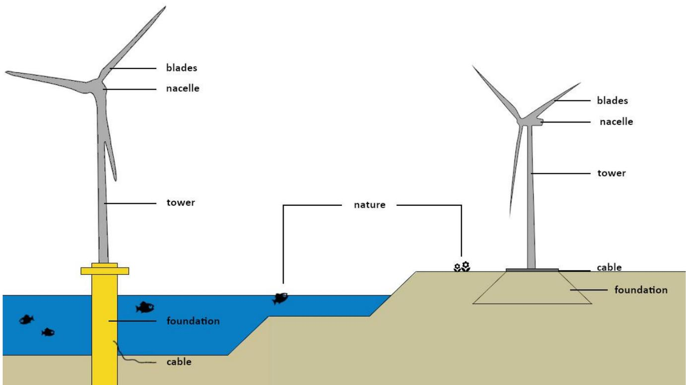
Figure 5: Schematic representation of structural elements of a wind turbine
